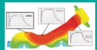
Temperature prediction correlation at thermocouple locations
